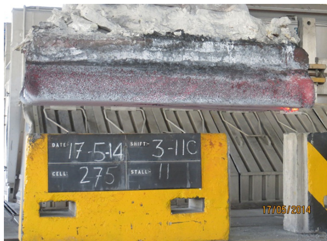
Figure 10. Anode spike from HRS pot.
